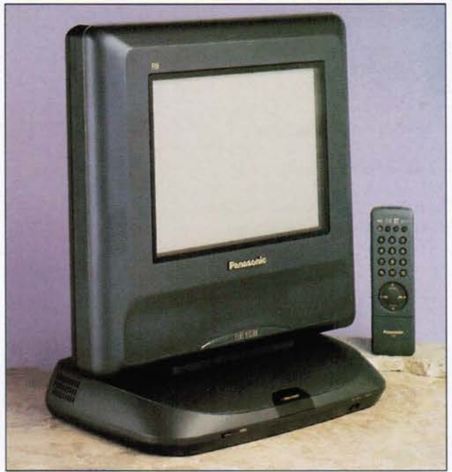
Fig. 7: 1994: Matsushita's Flat Vision TV – which was available very briefly in Japan – contained the company's flat "beam-matrix" tube, one of several attempts to make a commercially successful flat CRT.
